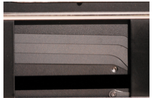
Vertical-travel focal-plane shutter firing at 1/500 of a second.
